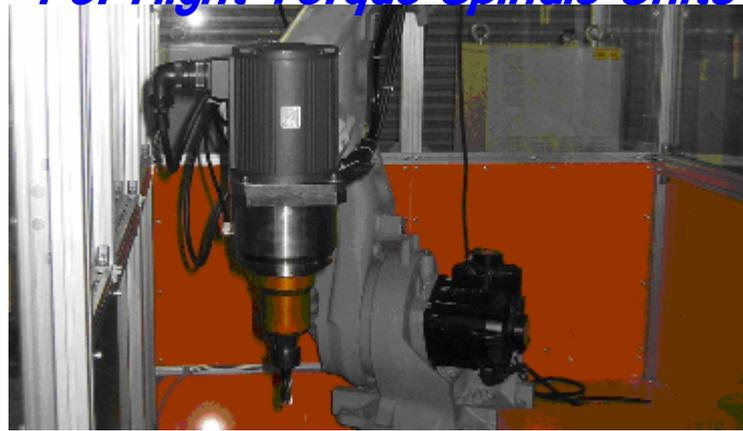
**Super Finish HiSP Quick Change System for High Torque Spindle Unit 主轴外形图**
